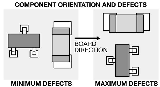
Figure 9. Component Orientation
